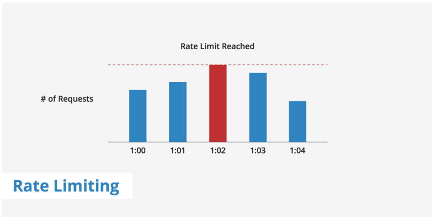
Fig. 2. Rate limit threshold detection and application of rate limiting [1].
