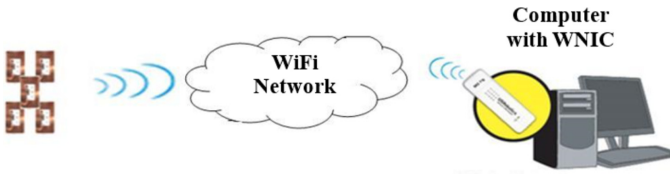
Fig. 4. The communication procedure through IEEE 802.11b between an RFID tag with the mapped EPC–IPv6 address structure and a computer with WNIC.
