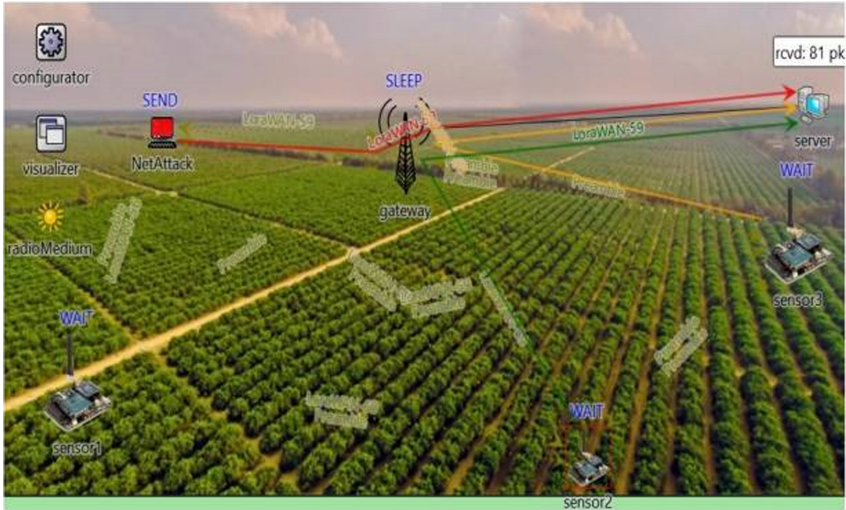
Fig. 5. The topology of WSN for monitoring of agriculture conditions [11].
