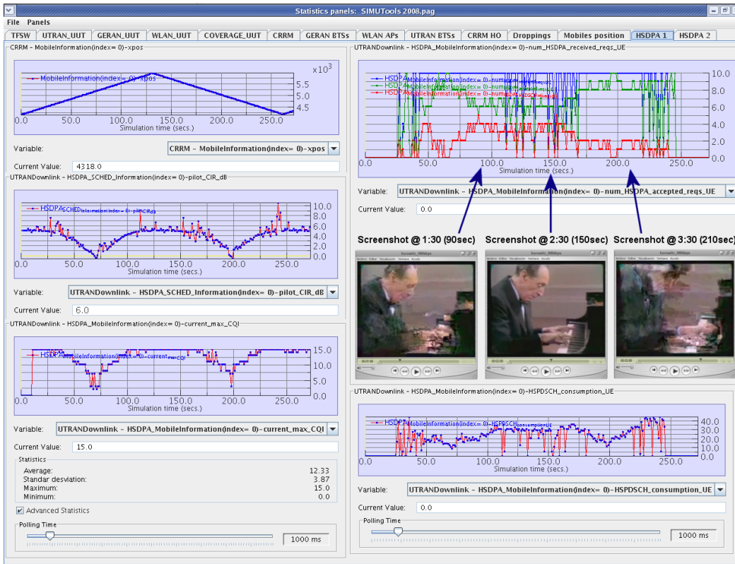
Figure 8: Real-time performance of the Round Robin scheduling criterion.
