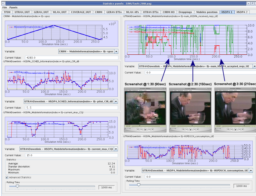
Figure 7: Real-time performance of the Maximum C/I scheduling criterion.
