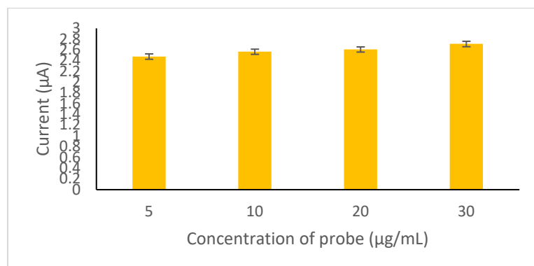
Figure 4. Determination of probe DNA concentration (5.0, 10.0, 20.0, 30.0 µg/mL) against the peak of the guanine oxidation current. Determination of current uses differential pulse voltammetry, scan rate 0.008 V/s in the potential range -0.2 V to +1.4 V. The target concentration for hybridization is 5.0 µg/mL.
