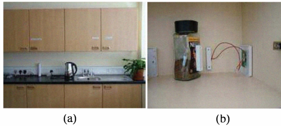
Figure 2. The smart kitchen laboratory in the University of Ulster at Jordanstown: (a) an overall kitchen view; (b) a coffee jar attached with a contact sensor
