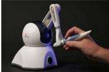
Figure 1. (a) PHANToM Omni 6DOF
