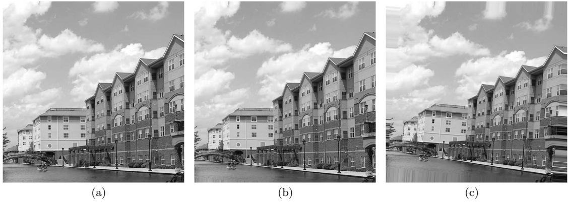
Figure 3: Geometric distortions in single cameras: (a) No distortion (b) Perspective (c) Planar(rotation)
