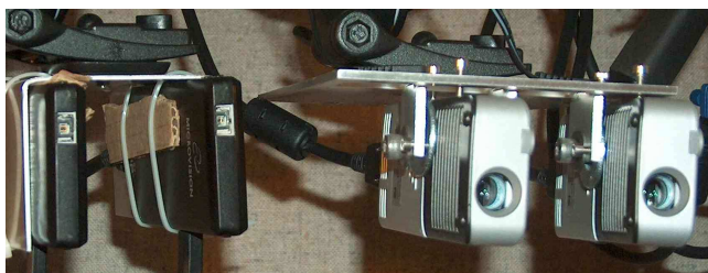
Figure 7. A pair of Microvision (left) and 3M (right) pico projectors assembled in a binocular stereo mode.
