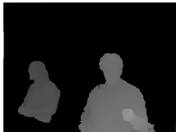
Figure 11 - Disparity fusion result: HRM trifocal combined with wide baseline result
