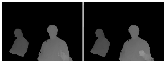
Figure 10 - Disparity images: Wide baseline (left), trifocal short baseline system (right)
