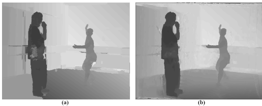
Figure 6: (a) Initial depth estimate, (b) refined depth map for Ballet .
