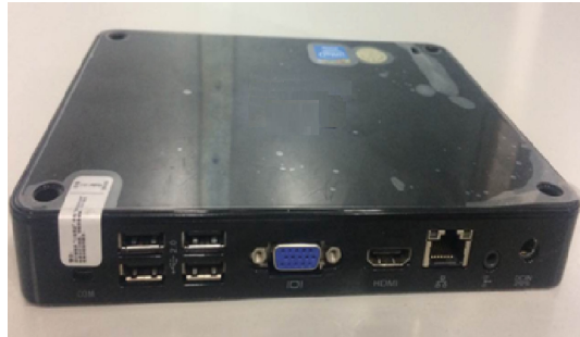
Fig. 5. Customized box to transmit data to control center
