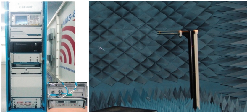
Fig. 6. Beidou OTA test system based on 8600 chamber
