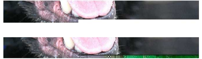
Figure 6: An example of an image corruption which can be revealed by decoding sectors one at the time. This image (of a dog) was taken from the 2007 DFRWS at header offset 87716 sectors. The top part is shown after decoding 243 sectors, while the bottom part was after decoding 244 sectors. The black bands illustrate the region over which the Estimate (Eq. 1) was taken. This region is restricted to the boundary between the smaller image and the image obtained by decoding more data.
