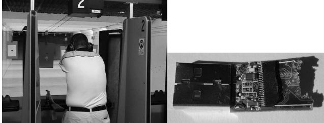
Figure 8: Left: a memory stick is shot with a pistol. Right: the remains of the memory stick. The 3 mm slice of chip is all that could be found of the Flash memory.
