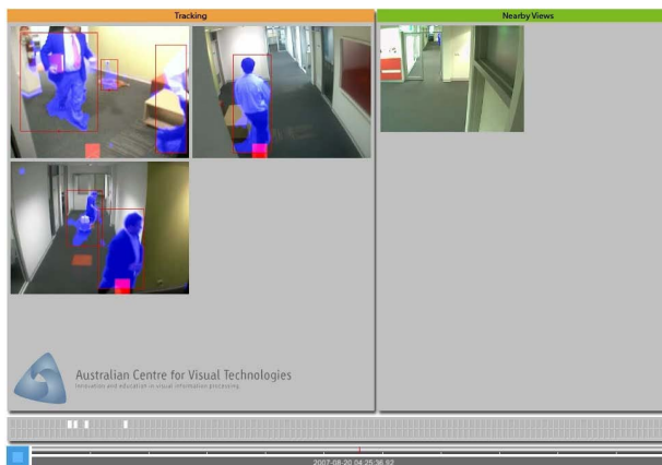
Figure 5: The system shows the cameras in which the target is believed to be present, along with a set of cameras where the camera may travel next. At any time, the user may override the system and request that tracking be restarted on any visible target.
