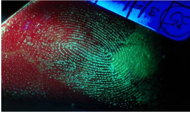
Figure 3. The UV light picture of the latent fingerprint developed by the cyanoacrylate fuming technique.
