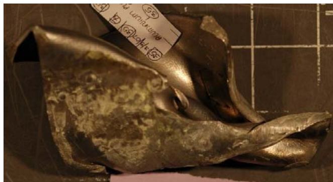
Figure 2. An aluminium plate after exposure to blast located 0.25 m away from 0.7 kg explosive charge.
