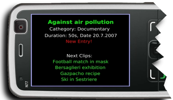
Figure 8 Mobile TV terminal with a frame of the title clip automatically generated for the VideoBlog.
