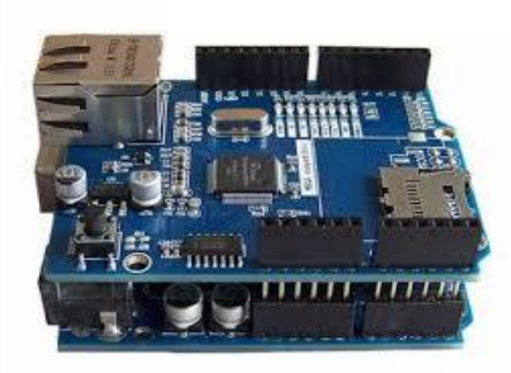
Gambar 2. Arduino with Ethernet Shield
