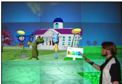
Figure 1. User inputs the number '1' ASL handshape with the cybergloves in response to a question asked by the 'lizard' character. SMILE in the background displayed on a 12-screen tiled wall
