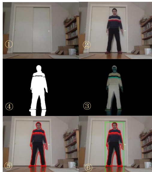
Fig. 5. ROI basic extraction processes
