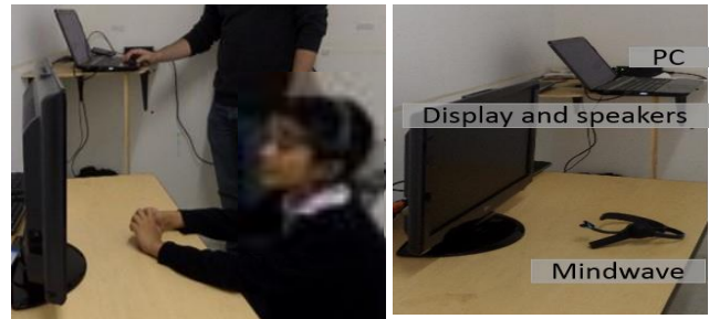
Figure 1. A child with autism hearing a sound and using the Mindwave headband during the study (left). Set-up of the study (right).
