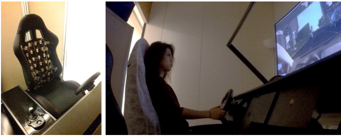
Figure 2. Driving simulator with vibrotactile seat (left) and while participant is experiencing fast breathing intervention (right).
