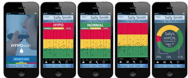
Figure 2. First iteration of the HYPOalert static interfaces. First interface displays the app splash-page. All remaining interfaces indicate the patient's name and reading date/time. Interfaces 2-4: (1) Three color-coded visualization areas: Green=NORMAL, Yellow=APPROACHING (or Caution), and Red=HYPO, and (2) Hourly indication of breathing times and their location on the HYPO visualization scale. Interface 4 displays the patient's weekly breathing summary, broken down in percentages.
