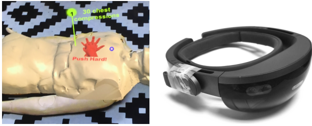
Figure 1. Envisioned MR prototype for expert-guided CPR. Left: chest compression instructions, and correct positioning of the hands displayed on top of a resuscitation mannequin. Right: Microsoft HoloLens head-mounted display; note the clicker taped to the head-mounted display as it was used for our experiment.
