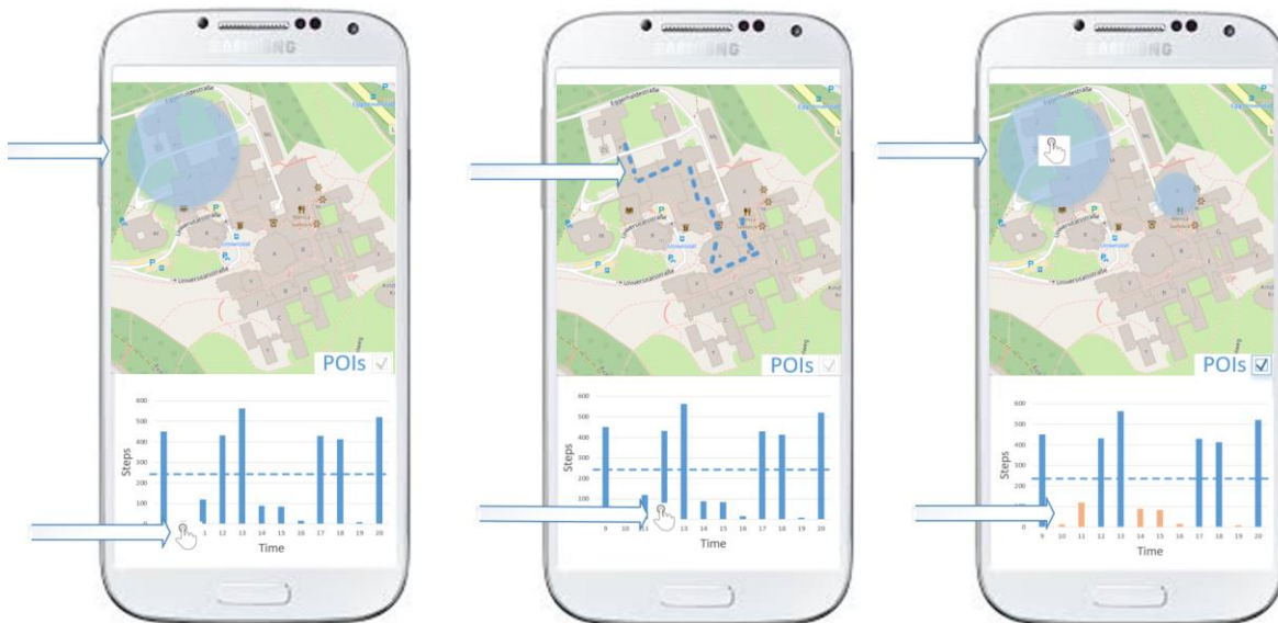
Figure 3: The interface of our mobility pattern visualization app. The corresponding POI shows up on the map when a sedentary hour bar is clicked in the bar chart (left). The corresponding route shows up on the map when an active hour bar is clicked in the bar chart (middle). The corresponding hours bars are highlighted when a POI is clicked on the map (right).
