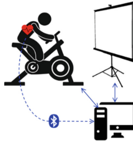
Fig. 1. The system setup. The dashed line represents Bluetooth connection; continuous line represents connections through cables.
