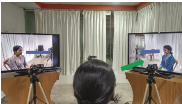
Fig. 3. A prototype system in action for a gaze aligned interactive consultation.
