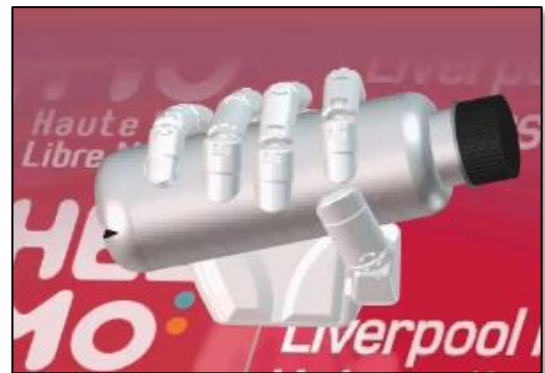
Figure 5. The robotic hand human-like grasping performance.
