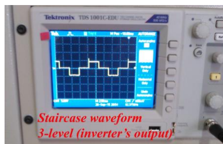
Fig. 13. Output waveform of the designed 3-level inverter.
