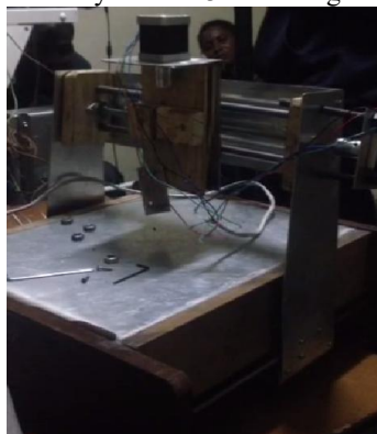
Figure 7: Cartesian robot during assembly
