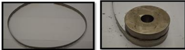
Fig. 3. Coiled green strips of Ti sponge at 0.3 mm roll gap and 5 rpm roll speed for set widths of 16 mm and 50 mm.
