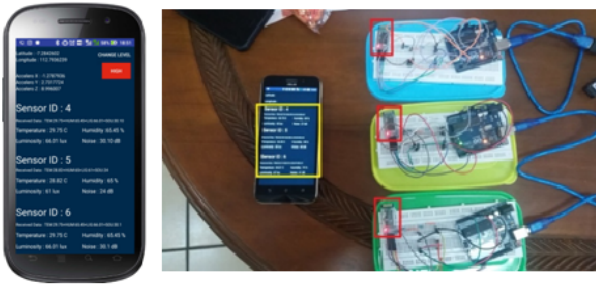
Figure 6: Basic Setup of a Mobile-IoT Crowdsensing Cluster with Three Arduino Boards
