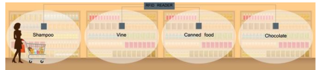
Figure 5: Principle of multiple antennas in the shopping center environment
