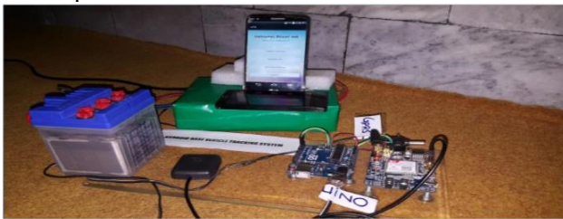
Fig. 9: Hardware implementation of vehicle tracking system
