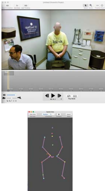
Figure 1: Body tracking data collected from a patient during a neurological assessment by the Kinect. Top: The patient here is shown sitting at rest prior to the start of the NIHSS examination. Bottom: Representation of the body through the Kinect v2 joints.
