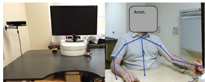
Figure 1. (Left) the haptic robot and Kinect sensor set up. (Right) a participant operating the haptic robot.
