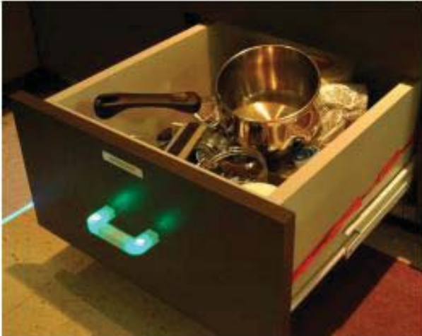
Figure 3: LED on Drawer Handle (from [17])
