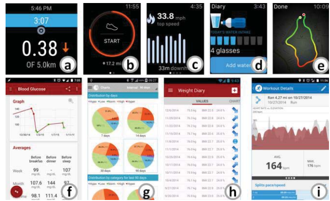
Figure 2.2 Common visualization techniques on smartwatch and smartphone applications. a) Text. b) Donut chart. c) Bar chart. d) Pictograph. e) Map. f) Line chart. g) Pie chart. h) Table. i) Complex visualization (e.g., 2D Area chart).
