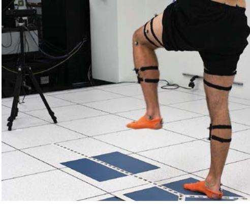
Figure 1. Subject performing a single leg stance trial in front of the Kinect (mounted on a tripod).
