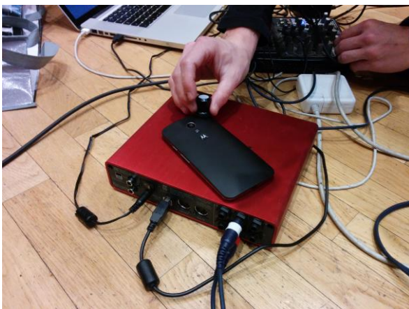
Figure 5. Using a pick-up coil to amplify the audio output of a smartphone
