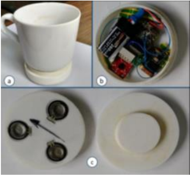
Figure 6: CogWatch coaster fitted under a mug (a) next to another dismantled coaster (b) and underside of coaster showing force sensitive resistors (c).
