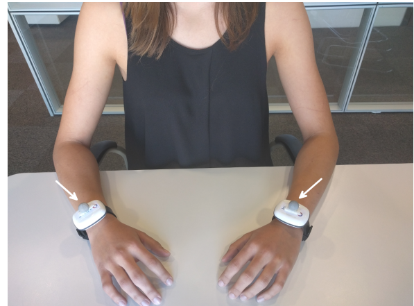
Figure 3. The markers put on the wristbands to be tracked through the Trio-OptiTrack.
