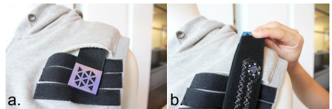
Figure 2. Sensors on ZISHI. (a)Front view of the elastic strap (b) IMU sensor embedded on the strap by conductive yarn.
