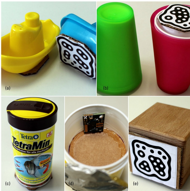
Figure 4. (a) Boat object; (b) "fish catcher"; (c) food can; (d) food can with IoT-acceleration sensor; (e) Navigation cube
