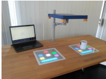
Figure 1: TagTrainer setup with three interactive surfaces.
