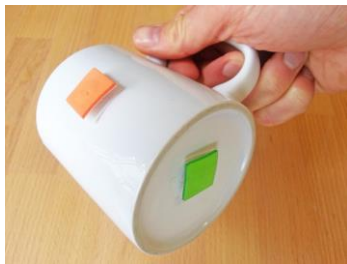
Figure 2: Two RFID tags have been attached to a cup. The tags allow TagTrainer to track the cup's position and rotation.
