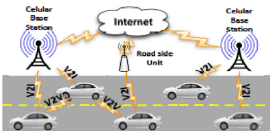
Figure 1. VANET communication architecture
