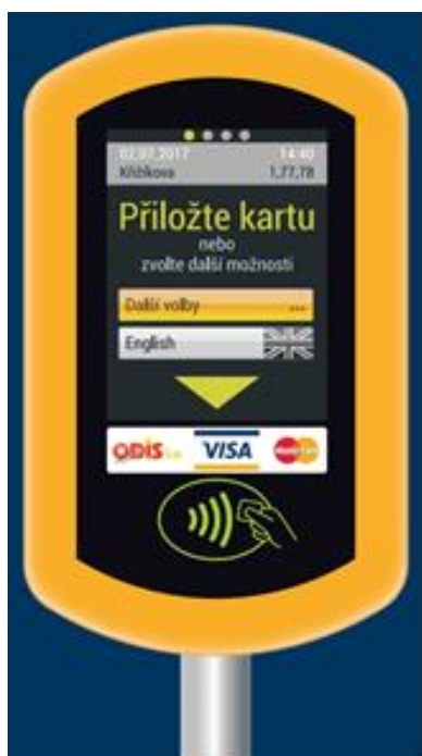
Figure 4. Terminal for contactless payment in public transport [ https://www.dpo.cz/soubory/aktuality/prirucky/platbni-karty-1.pdf ]
