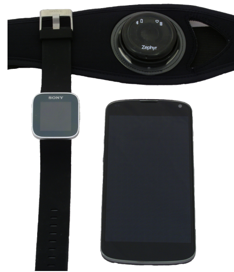
Figure 3. The apparatus: Zephyr BioHarness 3 (top), Sony SmartWatch (left) and LG Nexus 4 (right).
