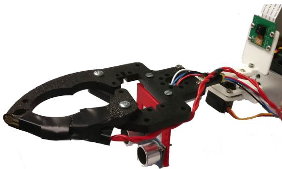
Figure 6. End effector with the camera module, force and proximity sensor
