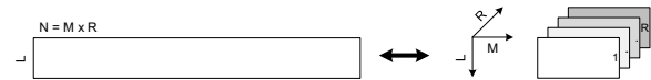
Figure 2: Interleaving original data block into subblocks to decouple circulant matrix size from ECG cycle length.
